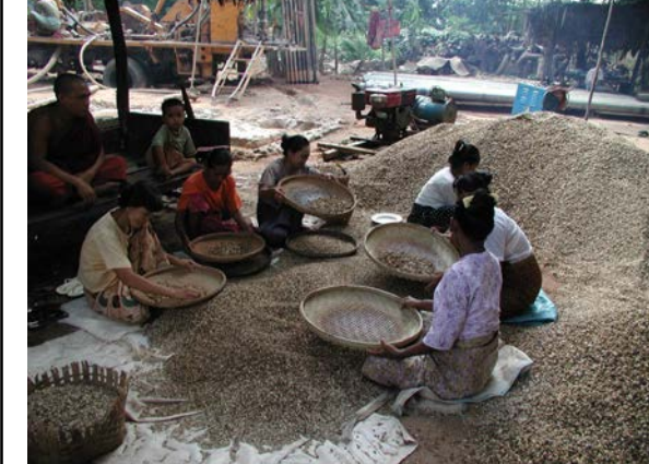
Selecting gravels by swiveling for gravel packing
