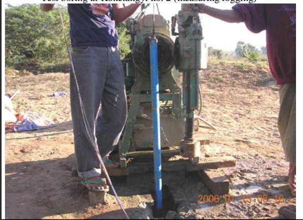
Test boring at Konetangyi no. 2 (measuring logging)
